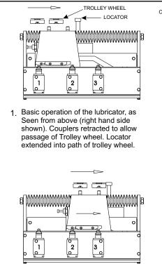
4. Couplers retracted upon completion of lubricant injection.
