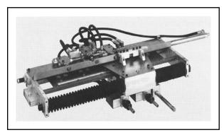
**Trolley Assemblies** – lubricant injector (coupler), load wheel locator, and controls to synchronize lubricator operation with conveyor movement.
