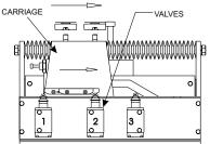
2. Trolley wheel contacts locator and Moves carriage assembly in direction of conveyor travel.
