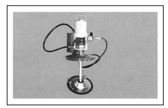
**Pump Assembly** – 50:1 pneumatically operated pump, container cover and follower plate, air inlet and grease outlet, and lube supply fault assembly.
