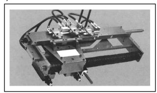
**Trolley Assembly** – lubricant injectors (couplers), side guide roller locator, and controls to synchronize lubricator operation with conveyor movement.
